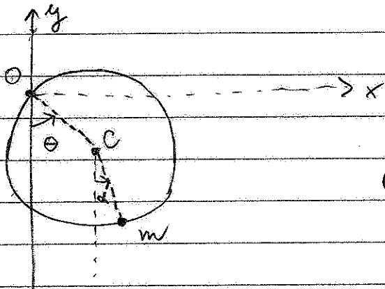
(i) The system has 2 d.o.f which we can parametrise using the angles  $\theta$ ,  $\alpha$  as in the figure
