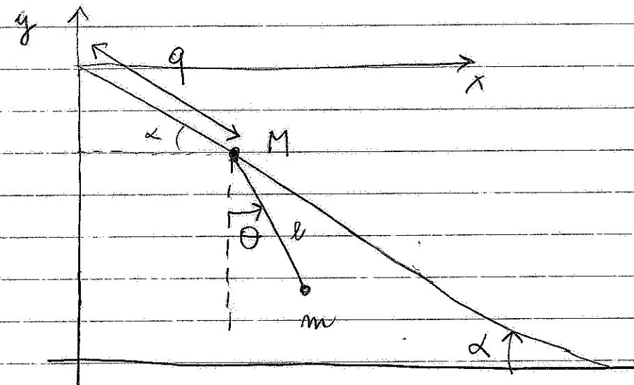
(i) 2 degrees of freedom - We can choose the position  $q$  of  $M$  measured along the inclined plane and the angle  $\theta$  as in the figure - '
