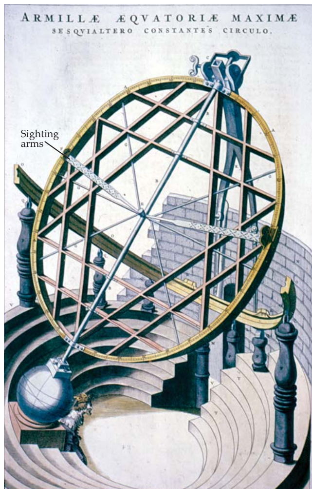
Figure 2. The equatorial armillary , Tycho's most impressive instrument, completed in 1585. The tilted axis running through the large (2.7-m wide) circle is parallel with Earth's axis. The circle is calibrated with 90^\circ at the poles and 0^\circ at the midpoint of its circumference. Two sighting arms establish the declination, the angular distance (north or south) of a star from the equator. Tycho could use one sighting arm to read the declination of a star or planet and then, in less than a minute's time, rotate the circle 180^\circ about the tilted axis to make a second independent determination with the other arm. (Published in 1662 and based on Tycho's original version, this illustration is by Willem Blaeu, a former assistant at Tycho's Hven observatory.)
