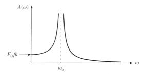
The important points to note are that there is divergence at the resonant frequency, that the function falls to zero at large frequency, and to a constant value at zero frequency
