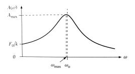
The main differences to not are that the function doesn't go to infinity, and that the peak position is a little lower than the resonant frequency.
