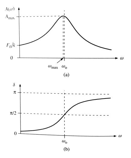
Let's work out the frequency at which the response is at a maximum – note that when we have no damping this is the natural frequency.
