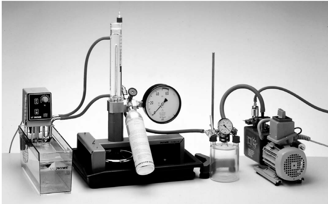
Fig. 1: Experimental set-up: Thermal equation of state and critical point.
