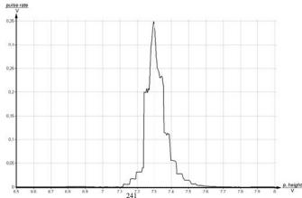
Fig. 3: Calibration measurement with open Americium source (E = 5.486 MeV).
