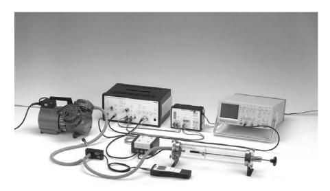
Fig. 1: Experimental set-up for  $\alpha$  particle spectroscopy.
