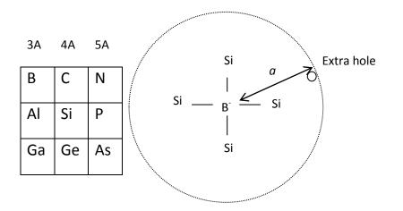
B<sup>-</sup> ion **accepts** one electron from the semiconductor, *p* increases relative to *n*, material is said to be **p-type and** the hole the **majority carrier**
