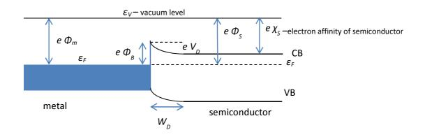
Electrons transfer to metal until Fermi levels are equalised which results in an electric field across  $W_D$  and in a diffusion potential  $V_D$ :
