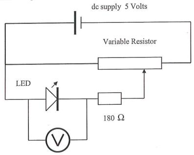
The 180  $\Omega$  resistor is there to protect the diode from damage. The variable enables you to adjust the voltage across the diode.
