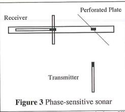
a complete phase shift of the same amount. The effect is seen more clearly if you switch to  $\overline{XY}$  display, where the pattern is sensitive to quite small movements of the perforated plate.
