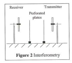
• Put the scope back into normal (not XY) two-beam operation, and move the perforated plates so as to measure the spacings of these maxima. This gives yet a third way of measuring the wavelength, so deduce it.
