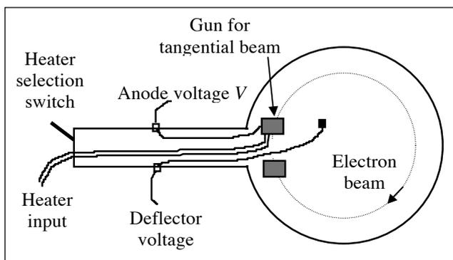
**Figure 1** Electron beam tube
