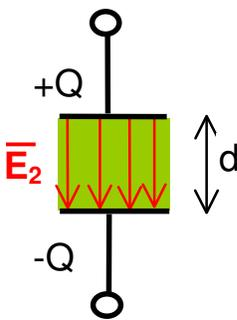
$$\text{With dielectric: } C_2 = \frac{Q}{\Delta V_2} = \frac{Q}{E_2 d} = \frac{KQ}{E_1 d} = \frac{K\epsilon_o A}{d}$$
