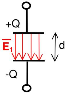
$$\text{No dielectric: } C_1 = \frac{Q}{\Delta V_1} = \frac{Q}{E_1 d} = \frac{\epsilon_o A}{d}$$
