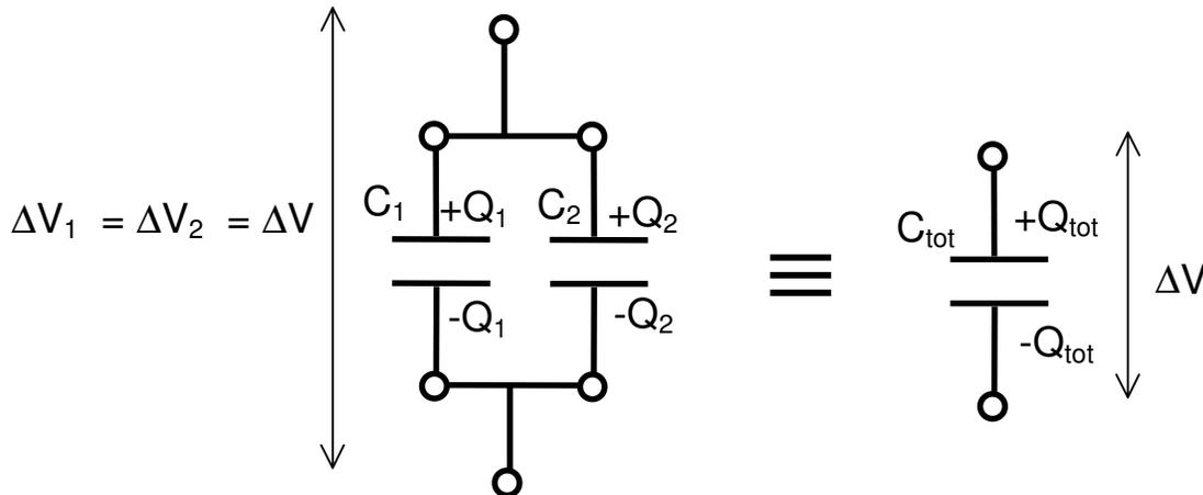
$$Q_{\text{tot}} = Q_1 + Q_2 \quad \Delta V_{\text{tot}} = \Delta V$$
