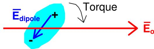
Even if no **INTRINSIC** dipoles exist, they can be **INDUCED** by an applied field  $\vec{E}_o$ , producing the same effect.
