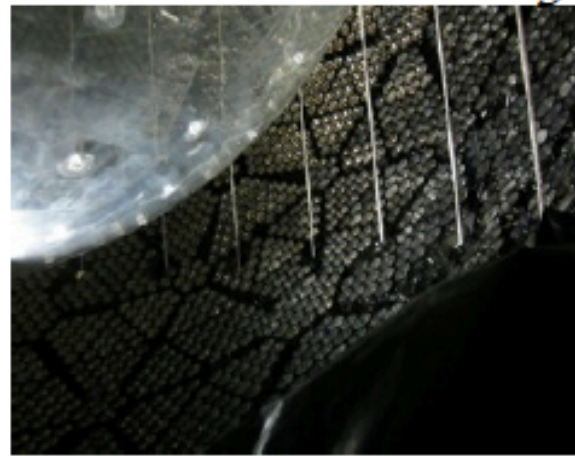
From GENIE lift, rope legs on opposite side passing through PSUP
